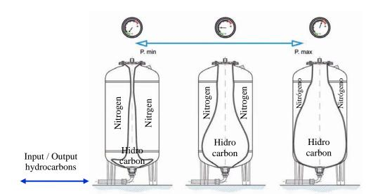
When the maximum desired pressure (pump stop pressure) is reached, the pressure switch cuts off the current and the oil circulation between the pump and the tank is interrupted at this moment. At this moment there will be a volume of oil stored inside the tank at a pressure equal to the pump stop pressure.
