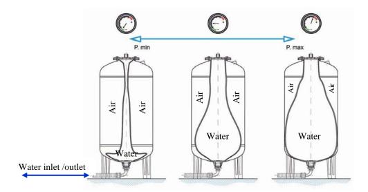
When the maximum required pressure is reached (pump stop pressure), the pressure switch cuts off the flow of water between the pump and AMR hydropneumatic tank. At this moment there will be a volume of water stored inside of the hydropneumatic tank at a pressure equal to the stopping pressure of the pump.
