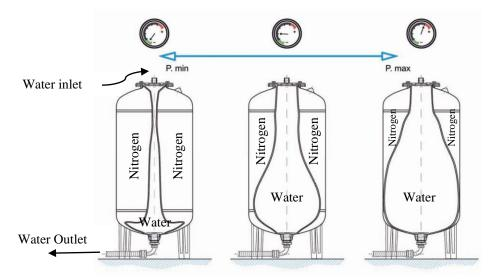
When the desired maximum pressure (pump stop pressure) is reached, the pressure switch cuts off the current and the water circulation between the pump and the tank is interrupted. At this point there will be a volume of water stored inside the tank at a pressure equal to the pump's shutdown pressure.
