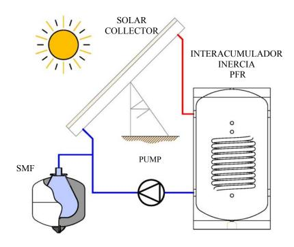
They are not suitable for use in open circuits with potable water or hydrocarbon fluids and those belonging to Group 1 in accordance with European Directive 2014/68/EU. The content of glycol in water should not exceed 50%. Vessels are not suitable for placement outdoors.
