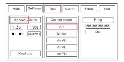
The solenoid valve is kept open by pressing the "Air" button. The container is completely discharged when the pressure on the display is zero and the air outlet has completely ceased. To perform larger service measures that require an internal examination, all fluid must also be emptied.
